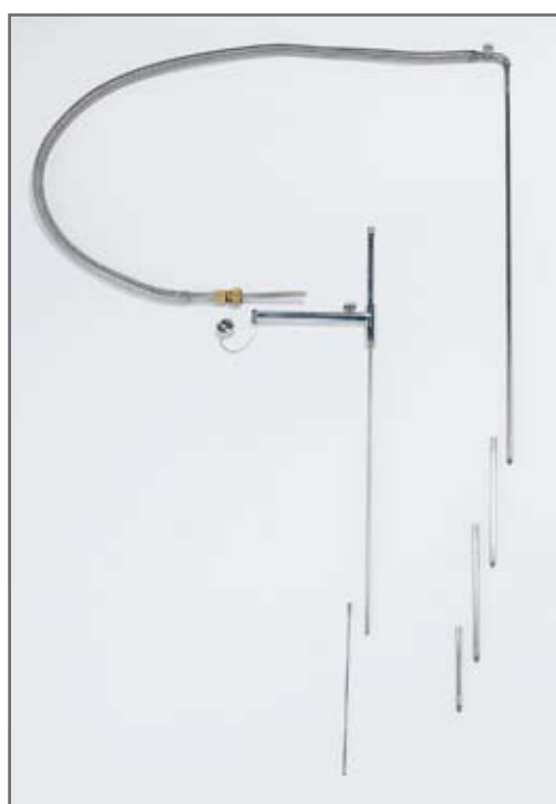
Left: Transfer pipe with "Oxford/Siemens male" coupling (left) and dip tube(right).
